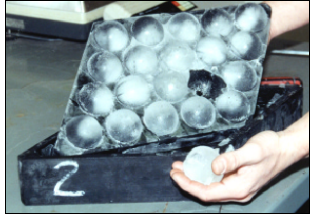
Figure 2. Solid ice stones made in rubber molds utilized for impact testing on roofing products.
