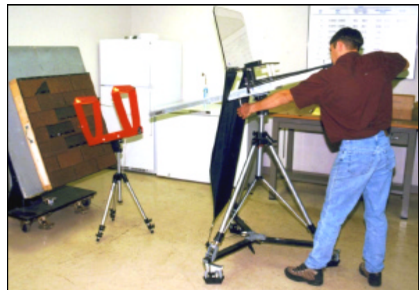
Figure 3. Ice ball launching (IBL) device with light sensors (chronograph) developed for impact testing.
